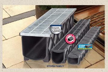
The brand new Storm Masta® is a large capacity surface water drainage system & is the perfect solution for collection of high surface water flows, in large domestic and light commercial applications. With a high intake class B galvanised steel grate, large 200mm channel depth/width, specially shaped self cleaning channel base, and multiple outlets for 150mm PVC stormwater pipe, Storm Masta® is designed to efficiently clear high flows of stormwater
